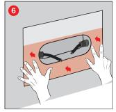
Press the lower part of the adhesive collar firmly into place.
