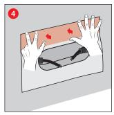
Press the upper part of the adhesive collar firmly into place.
