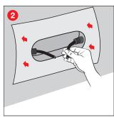
Cut the cable at an angle and pierce through the membrane of the integrated SEALplugs.
