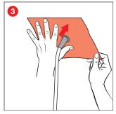
Press the adhesive collar firmly into place.
