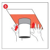
Press on the lower part of the adhesive collar firmly.
